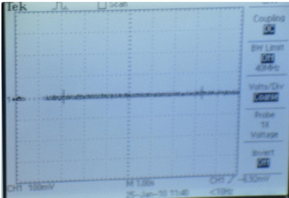
One of the problems which we encountered was that the AC line in had noise which was getting transferred to the bulb and which made it flicker thus sending a lot of spikes to the scope. This can be stopped by having a better regulated power supply.
