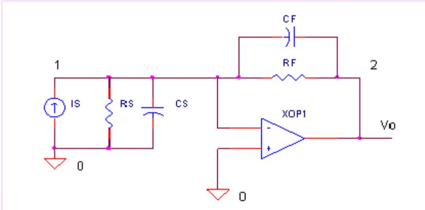
Figure 10 – Trans-impedance amplifier
