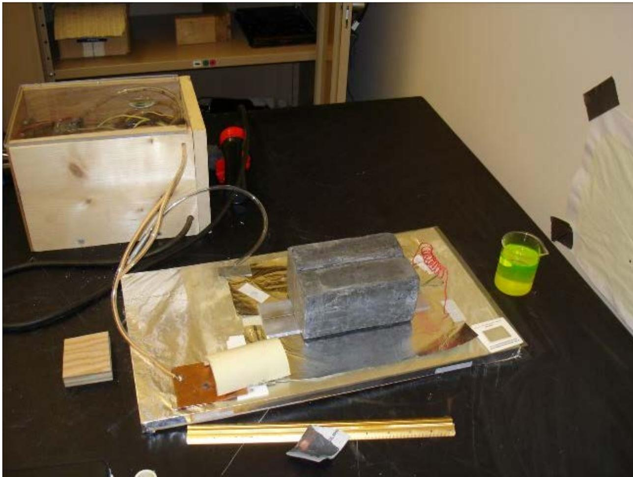
The TEA laser and power supply. The power supply is contained in the box at the top left. The laser capacitor consists of the aluminum foil and transparencies wrapped around the shelf board. The laser discharge path is formed by the two strips of aluminum underneath the two lead bricks. The spark gap is housed underneath the plastic tube at the bottom.
