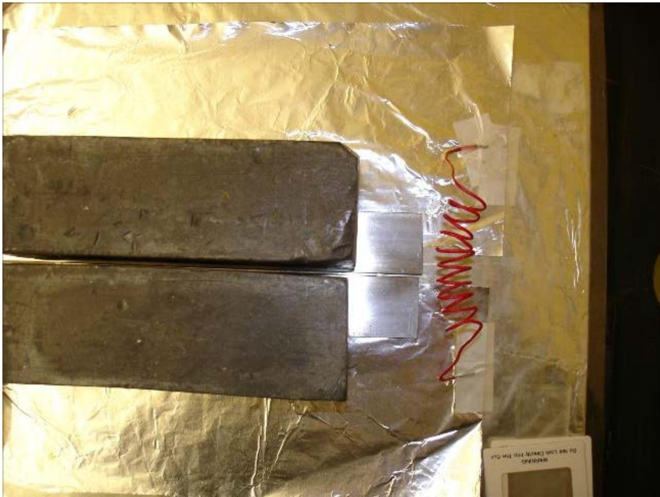
The laser discharge path. Each lead brick rests on a separate aluminum strip. The spark between the aluminum strips provides the energy to power the laser. Each aluminum strip is about 2cm wide. The red inductor permits both capacitor plates to charge and forces the charge to flow through the gap when the capacitor discharges. The diffraction grating at the bottom right was used to measure the wavelength of the laser light.
