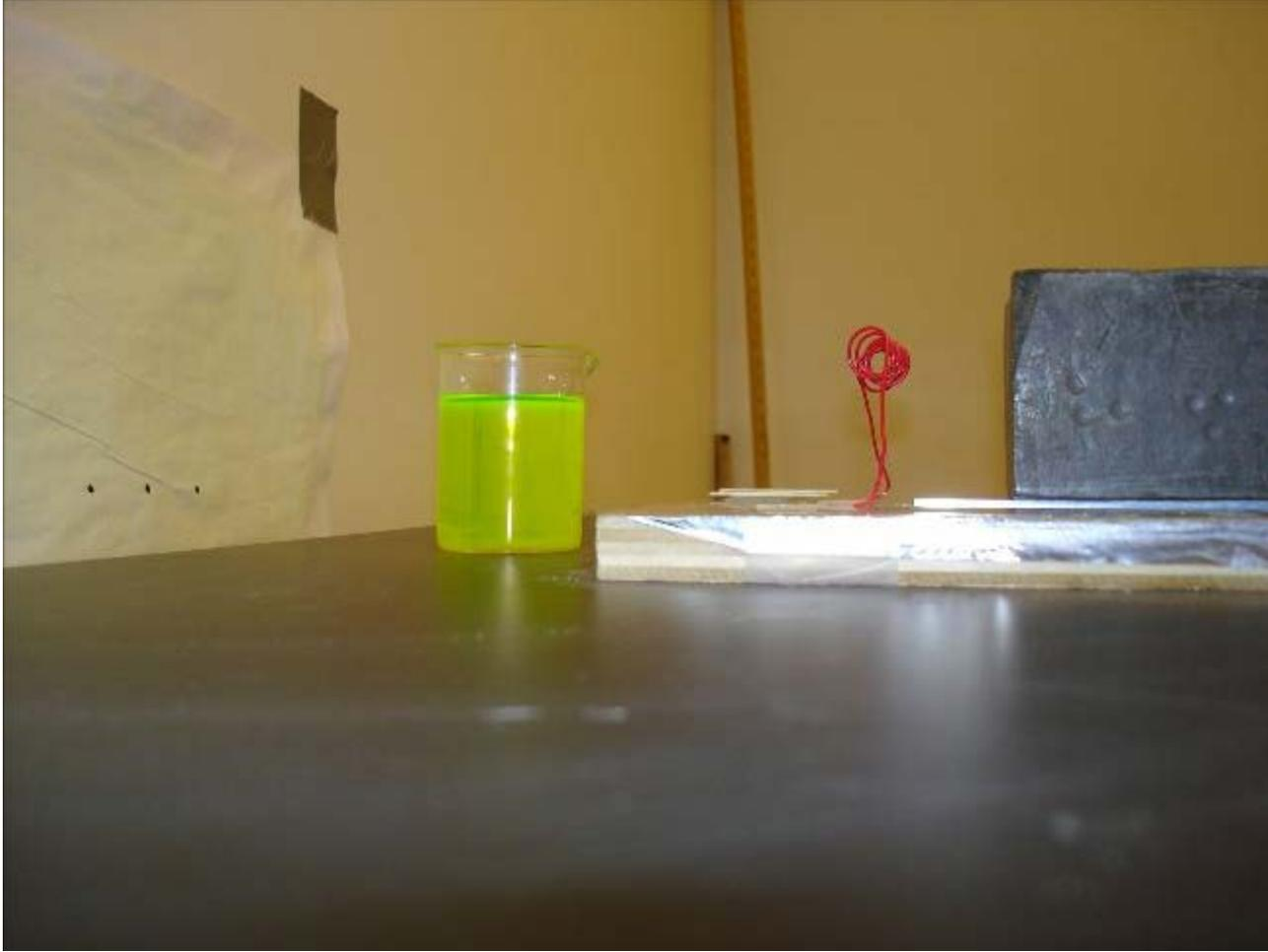
The laser is all set to fire. The laser is pointed at a beaker of fluorescent dye. When the laser fires, the beam will make the dye glow. The dots on the wall show the positions of the laser beam after it passed through a diffraction grating.
