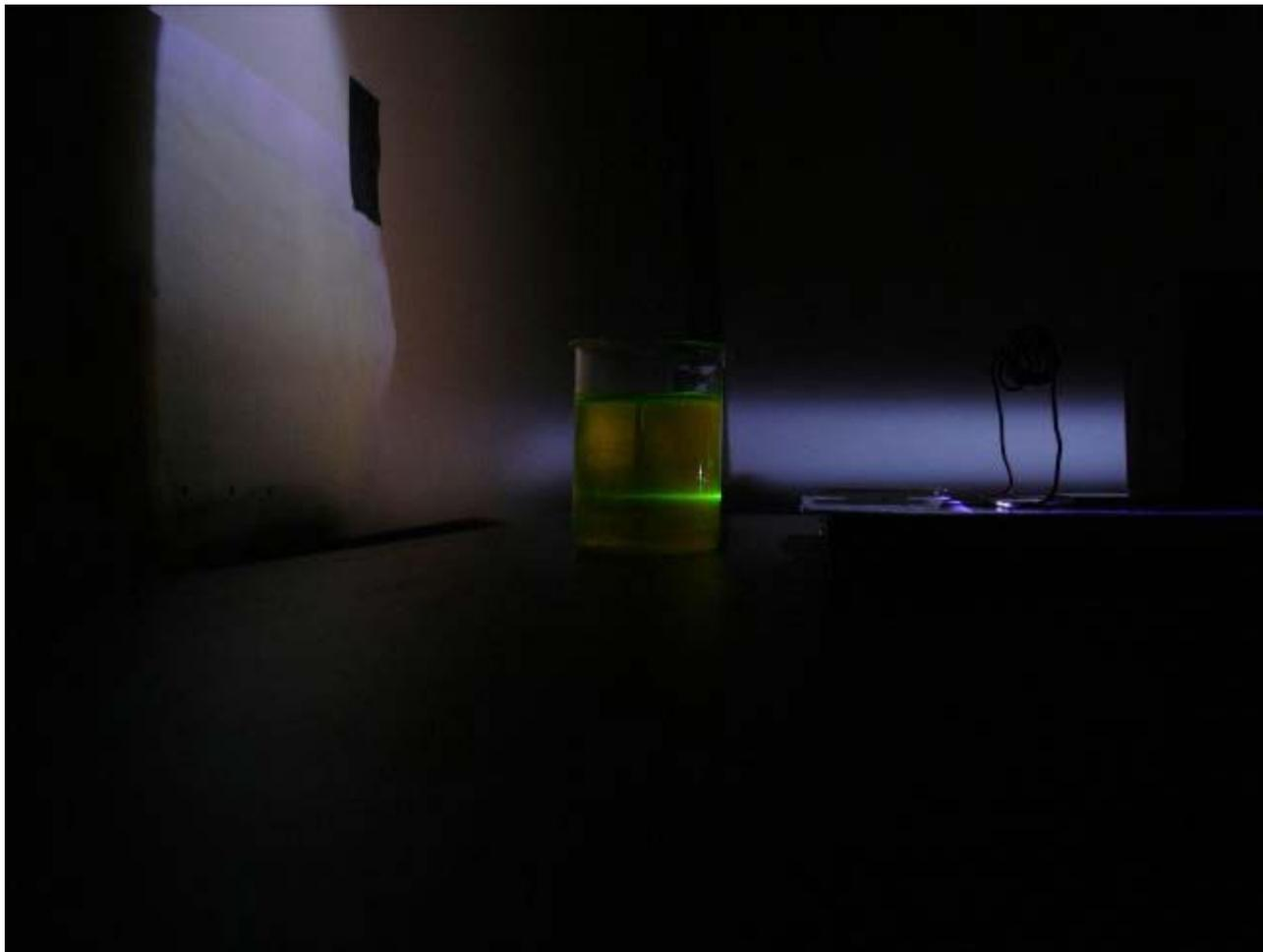
The laser is firing. The thin, bright green streak of light in the beaker is due to the laser. The purple glow near the laser is due to the spark gap.
