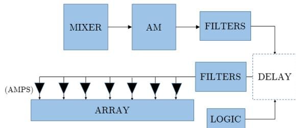
FIG. 4. Block diagram for complete array
