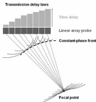
FIG. 1. Simplified implementation of a TTD phased array
