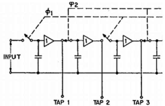
FIG. 3. Equivalent circuit for simple bucket brigade device
