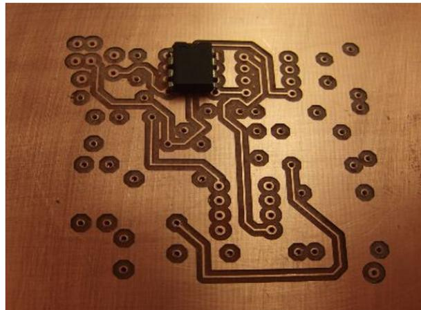
FIG. 5. One side of the modulator module, milled onto a copper clad
