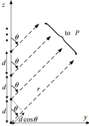
FIG. 2. Illustration of  $N$  element array
