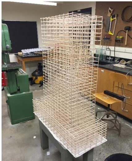
Figure 2: Scaled model of the building made of balsawood.
