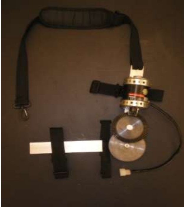
Figure 10. The exoskeleton of my left arm with one degree of freedom.
