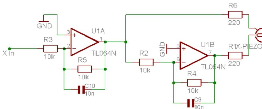
Figure 7: Supply for x-piezo. Supply for y-piezo is identical.
