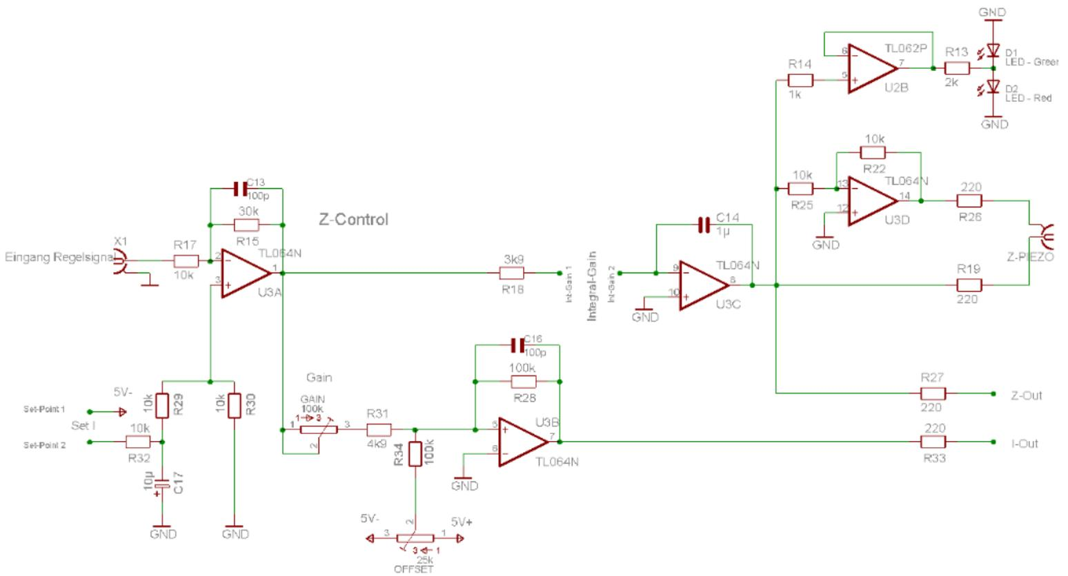
Figure 8: Supply and control for z-piezo.
