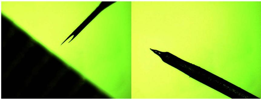
Left Image: Bifurcated tip caused by using the snips to cut the original wire.
