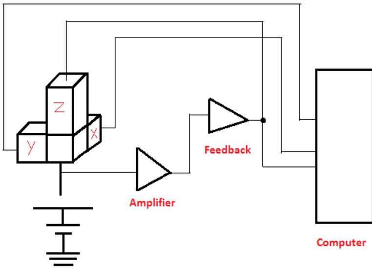
*Figure 3: Block diagram of a STM*
