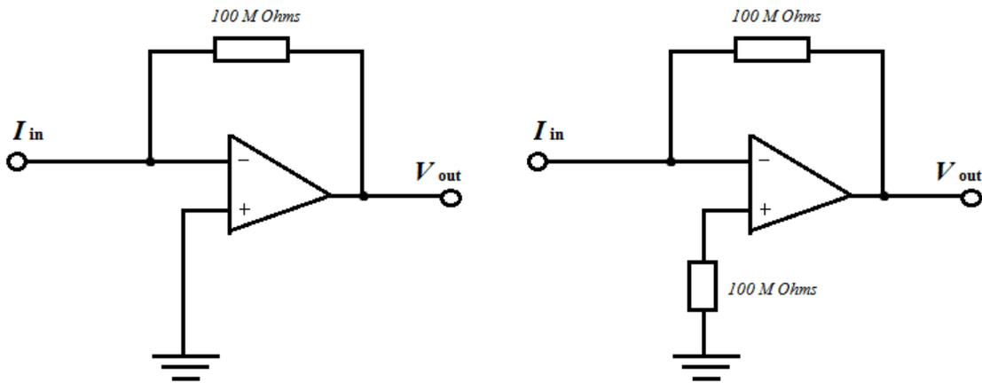
Figure 6: Simple I-V converter pre-amp (left) and modified design (right). Offset circuitry not shown.
