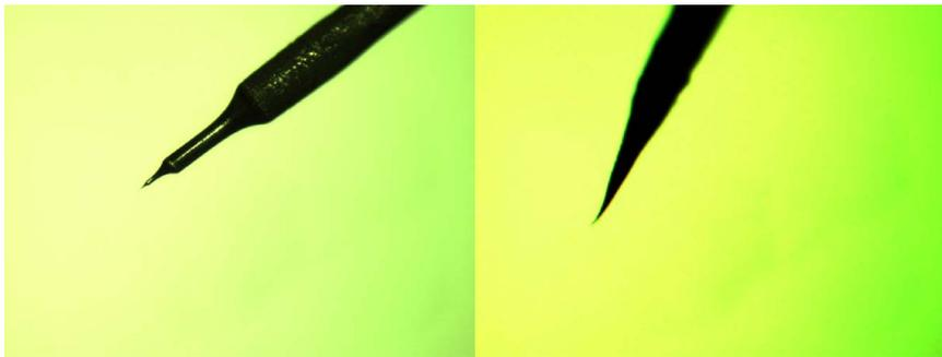
Left Image: Example of a multistage tip caused by shifting of the meniscus.
