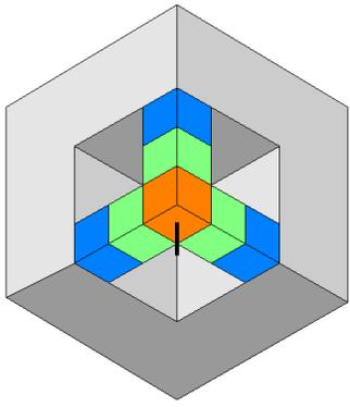
*STM scanning head schematic. Brass cube in orange; crystal beads in green; piezo controllers in blue; aluminum block in gray.*
