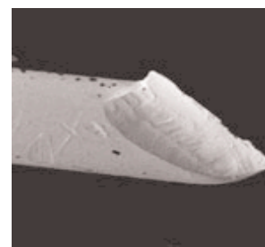
Figures 13 and 14: Etched and cut tips
