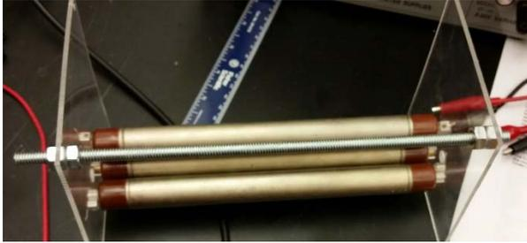
Figure 7: Three Geiger tubes suspended between plexiglass sheets
