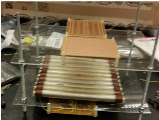
Figure 10d: Placement of second row of Geiger tubes
